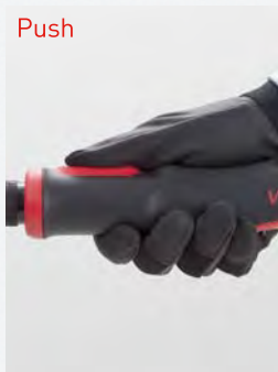
Push method for horizontal driving
