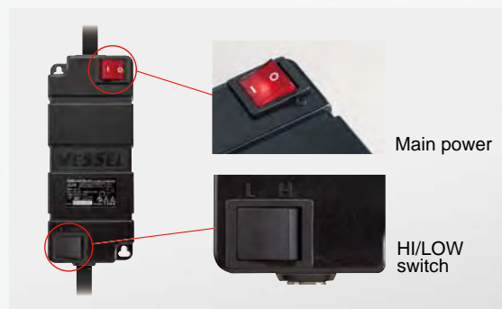
External controller capable of HI or LOW selection
