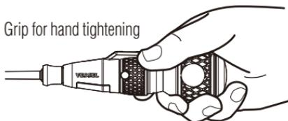
**⚠ CAUTION: Do not slide the switch while the spindle is locked and the screw is manually tightened.** The power tool may be damaged.
