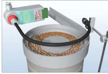
Vibratory bowl feeder (joint nozzle + shower tube)
